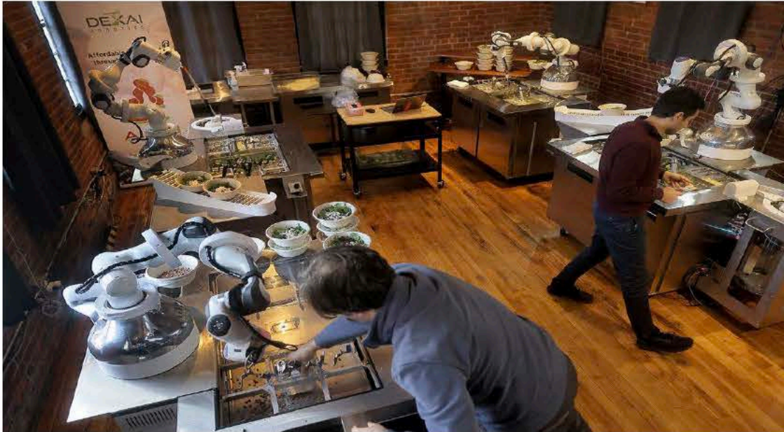
Dexai's robot dubbed "Alfred" is a food safe-certified robotic arm that can sit in front of a row of hotel pans of ingredients, and uses traditional kitchen utensils like scoops and tongs. Photo courtesy Lane Turner/Boston Globe
