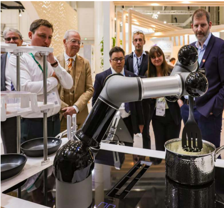
data—one of the world’s largest air and travel services providers—has implemented Moley Robotics’ AI-powered cooking robot into its catering operations, serving identical dishes at scale. With advanced machine learning capabilities, it can recreate recipes by following pre-recorded chef instructions. It is also equipped with multiple sensors that enables it to precisely measure ingredients and execute complex cooking techniques. On top of that, the robot ensures consistent quality and good food hygiene. It can also quickly adapt to changes in real time. Photo courtesy Ulrich Perrey
